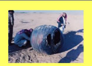
On 21 January 2001, a Delta 2 third stage, known as a PAM-D (Payload Assist Module - Delta), reentered the atmosphere over the Middle East. The titanium motor casing of the PAM-D, weighing about 70 kg, landed in Saudi Arabia. [Source: NASA]
